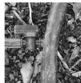
1/2" ball valve outlet tee (have to shorten barb).
